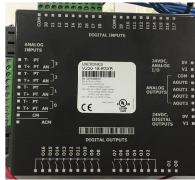
Figure 7: Unitronics Input-Output module
